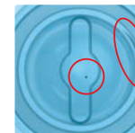
Shape B: foreign material and deformation
