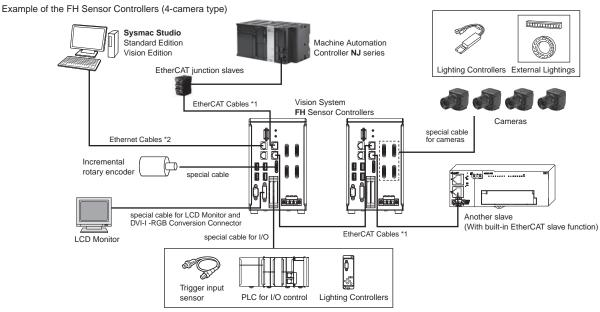
\*1. To use STP (shielded twisted-pair) cable of category 5 or higher with double shielding (braiding and aluminum foil tape) for EtherCAT and RJ45 connector.
